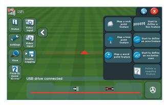
To configure the mapping options for warning zone distance and recording position, tap , tap and then tap . Set the mapping preferences for point, line, or area.
